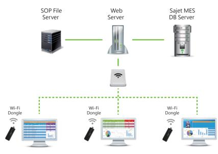
The new generation of Chroma eKanban solution integrates HDMI interface and different kinds of digital display monitors under Android platform. It helps to deliver real-time information to display monitors through Wi-Fi in factories. Moreover, it is easy to set up the layout configuration on Web interface so as to upload and broadcast real-time kanban information to factories, hospitals, retail stores, and public environments, providing the best choice of visual management solution.
